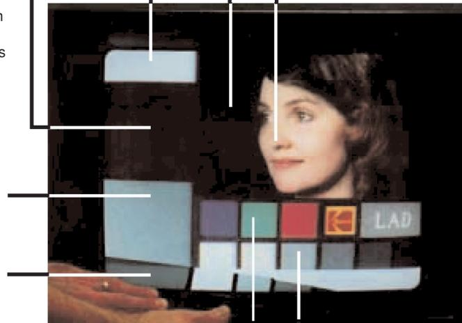
In the Laboratory Aim Density (LAD) printing control method, a standard control patch specifies densities midway between the minimum and maximum of those typically obtained for a normal camera exposure.
