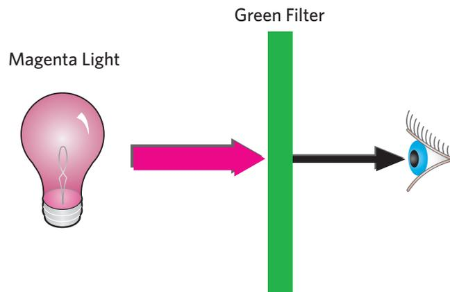
By adjusting a filter's intensity, we control the amount of light passing through it. An intense green filter absorbs practically all magenta light. As intensity diminishes, more magenta light passes through. Filtration is used to control the color of light during exposure and projection of film.
