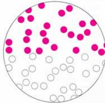
The silver developed by the first developer and the color developer has been removed, leaving only the magenta dye.
