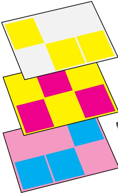
This negative was prepared from colored couplers. The unused yellowish coupler in the middle layer makes the magenta dye image apparent only through the green filter, and the unused reddish coupler in the bottom layer makes the cyan dye image apparent only through the red filter. Thus blue, green, and red light are controlled independently by the yellow, magenta, and cyan dyes, respectively. The dye images do not interfere with each other to cause errors in color prints.
