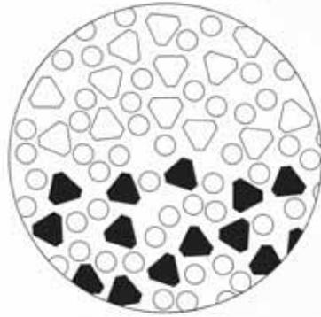
In the lower half of the circle, the first developer has reduced the silver halide crystals to metallic silver.
