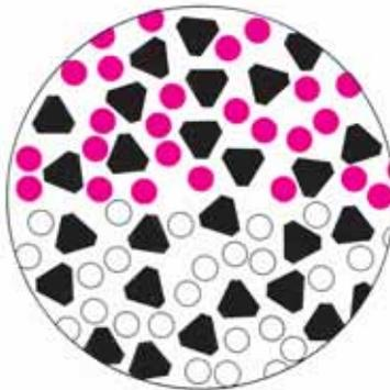
In the upper half of the circle, oxidized color developer has combined with the coupler in the carrier.
