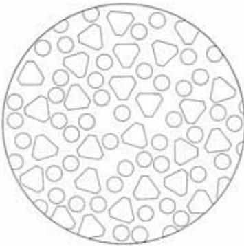
Diagram of Ektachrome film emulsion, showing crystals of silver halide and globules of carrier dispersed in gelatin.
