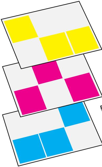
The color negative below was prepared from colorless couplers. At the left are the three emulsion layers as they would appear if they could be peeled apart. Examine the layers through KODAK WRATTEN No. 29 (red), No. 61 (green), and No. 47 (blue) Filters. If the dyes forming the images were perfect, each image would be visible only through the complementary filter. Actually, the magenta image is also visible through the blue filter, and the cyan image is visible through all three filters.
