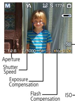
**Aperture**—also known as f-stop or f-number, controls the size of the lens opening, which determines the depth of field. Smaller f-numbers, for example f/2.8, refer to a bigger lens opening. Larger f-numbers, for example f/8, refer to a smaller lens opening. Larger f-numbers keep the main subject sharp; good for landscapes and well-lit conditions. Smaller f-numbers are good for portraits and low-light conditions. The highest and lowest aperture numbers may be affected by optical zoom.
