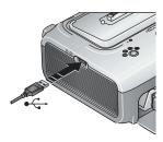
1 Using the USB cable for the PictBridge device, plug the USB connector from the PictBridge device into the USB connector located on the side of the printer dock.
