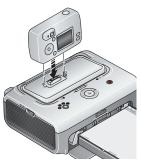
**3** Place the camera in the printer dock, making sure to align the dock connector and locator hole with the camera connector and locator pin. Push down to seat the connector.
