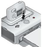
**3** Press and hold the Battery charging lights/Refresh button, until the Battery charging lights begin flashing green (approximately 5 seconds).
