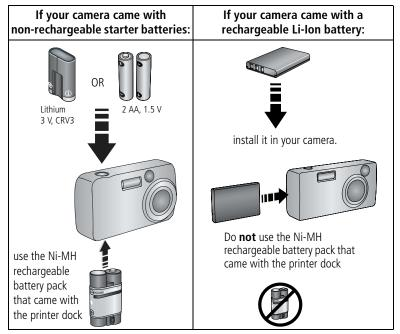
NOTE: The Ni-MH rechargeable battery pack and Li-Ion rechargeable battery are not charged when you receive them. Make sure to completely charge them before using them with your camera (see page 10).
