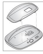
Use custom camera insert (included with camera). If unavailable, use universal camera insert (included with Camera Dock).
