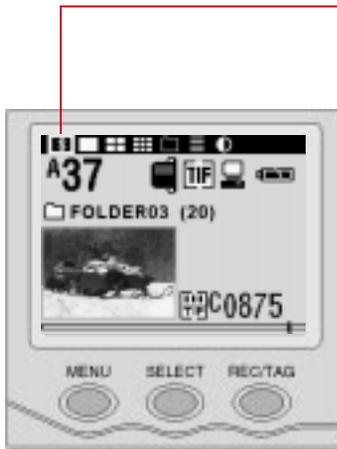
**1** Press and hold the MENU button and rotate the Main-Command dial to highlight the Status icon.
