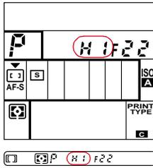
➔ If **HI** appears in the shutter speed position—Over-exposure alert: Use a Nikon ND or similar filter.
