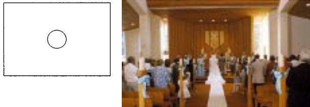
Nearly 100% of the meter's sensitivity is concentrated on the 2.5 mm-diameter circle (approximately 1% of entire frame) in the center of the viewfinder. Use this meter for extra-selective exposure control; experience is required to achieve optimum results.
