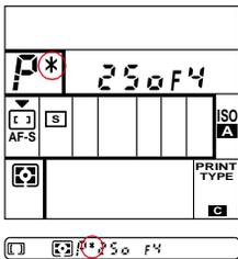
The shutter speed/aperture combinations available may be limited due to subject brightness. To indicate the program has been shifted, the Flexible Program indicator (\*) appears beside the Auto-Multi Program or the Vari-Program indication on the Camera Status LCD panel.
