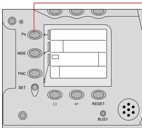
Press and hold the Ps button and rotate the Main-Command dial until the desired Vari-Program symbol (page 6-4) appears in the Camera Status LCD panel.
