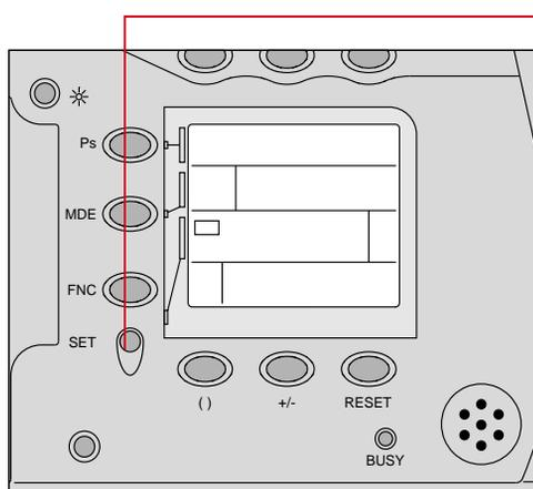
**3** Press and hold the SET button and rotate the Main-Command dial until the desired flash symbol appears.
