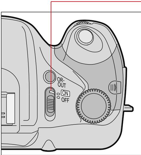
Slide the Power switch to On to turn the camera On.
