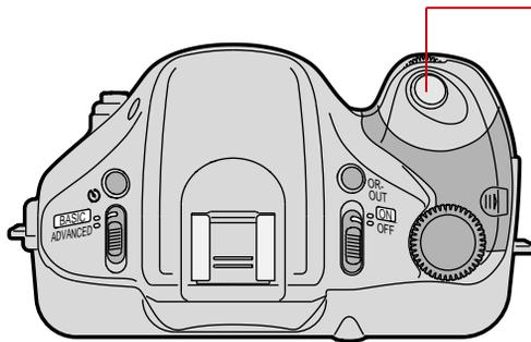
Firmly pressing the Shutter Release button captures an image.
