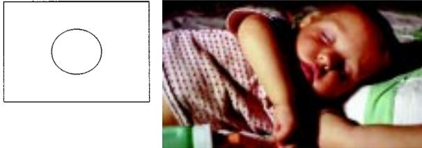
With approximately 65% of the meter's sensitivity concentrated on the 8.4 mm-diameter circle in the viewfinder and approximately 35% outside this circle, this meter is useful when you want to base your exposure on a specific area in the scene. In Auto Exposure mode, to measure the brightness of the picture's off-center portion, use the AE-L button. Refer to "Using the Auto Exposure Lock Function" on page 7-4.
