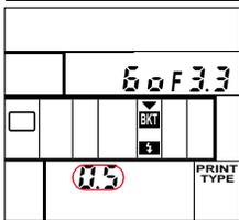
**3** Press and hold the SET button and rotate the Main-Command dial until the desired compensation degree (**0.5** or **1.0**) appears.
