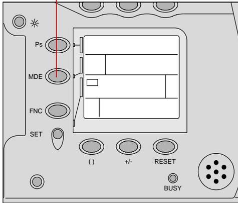
Press and hold the MDE button, and rotate the Main-Command dial to set **P** for Auto-Multi Program, **S** for Shutter-Priority Auto, **A** for Aperture-Priority Auto, or **M** for Manual.
