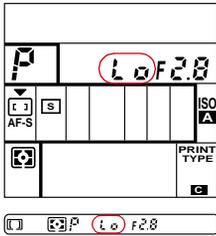
➔ If **Lo** appears in the shutter speed position—Under-exposure alert: Use built-in flash or a Nikon Speedlight.
