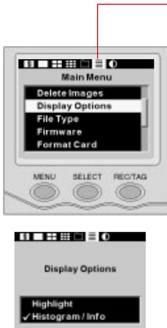
**1** Press the MENU button to turn the Image LCD panel On.
