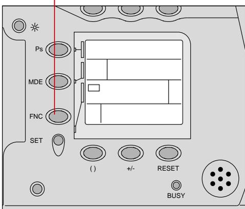
To confirm the compensation value in the Camera Status LCD panel, press and hold the FNC button and rotate the Main-Command dial until the Function Set indicator (▼) appears and
