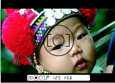
Lightly press the Shutter Release button to start the autofocus operation. During the operation, ◀ or ▶ (for front or rear focus) may appear. When the subject is in focus, a ● appears in the viewfinder.
