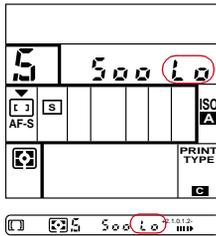
➡ If **Lo** appears with the electronic analog display (lower right corner of viewfinder)\*—Under-exposure alert: Select a slower shutter speed or use the built-in flash or a Nikon Speedlight.
