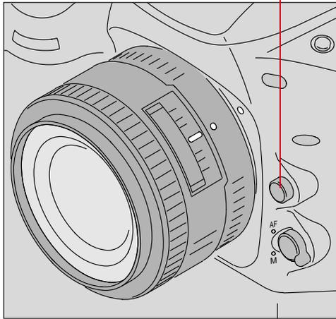
Press and hold the Lens Release button, then turn the lens clockwise.
