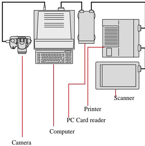
➤ You may connect more than one camera or other 1394 devices to the card as long as you avoid a closed loop configuration. (The drawing is an example of an acceptable configuration.)
