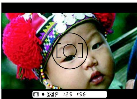
Confirm that the in-focus indicator (●), shutter speed and aperture indications appear in the viewfinder LCD.
