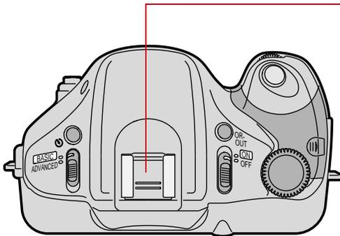
The ISO-type hot shoe allows direct mounting of a wide range of Nikon dedicated, electronic Speedlights. Refer to “Using Accessory Nikon Speedlights” on page 8-23.
