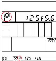
If the exposure meter and LCD indications automatically turn Off, turn them On again by lightly pressing the Shutter Release button.
