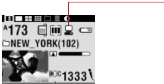
The Host Computer Connected icon on the Status screen appears when a valid cable connection is made. It flashes when a host computer application (such as the Kodak Software) is running.
