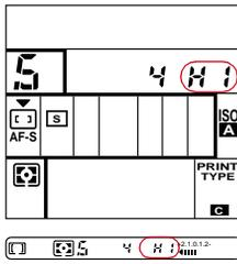
➡ If **HI** appears with the electronic analog display (lower right corner of viewfinder)\*—Over-exposure alert: Select a higher shutter speed or use a Nikon ND filter.
