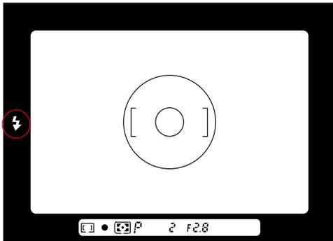
If a green ⚡ mark appears—Flash photography recommended: Available light is insufficient. Use the built-in flash or a Nikon Speedlight.
