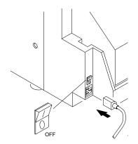
1. Check that the power switch is turned off  $(\bigcirc)$ .
