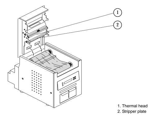
Internal View with Ribbon Installed
