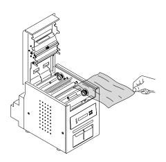
3. Remove the packing material.
