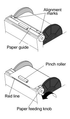
6. Align the edge of the paper with the alignment marks on the paper guide.
