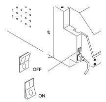
1. Press the power switch to on ( | ).
