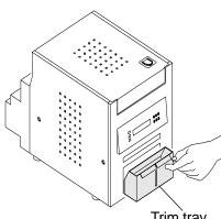
The trim tray collects paper trimmings that are generated when the printer cuts the prints.
