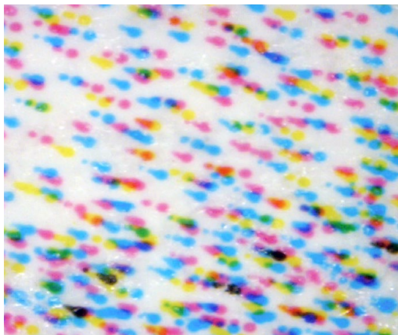
Figure 3: Microscopic view of droplets placed by KODAK Stream Inkjet Technology Printheads (left) compared to a competitive inkjet method (right)
