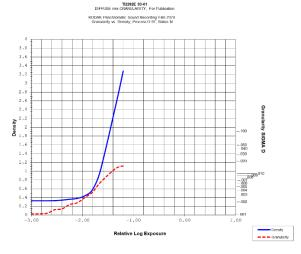
Read at a net diffuse visual density of 1.0 using a 48-micrometer aperture. **Note:** To find the rms Granularity for a given density, find the density on the left vertical scale and follow horizontally to the characteristic curve and then go vertically (up or down) to the granularity curve. At that point, follow horizontally to the Granularity Sigma D scale on the right. Read the number and multiply by 1000 for the rms value.
