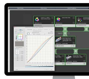
COLORFLOW Pro Software automatically generates G7 curves for consistent, quality color.
