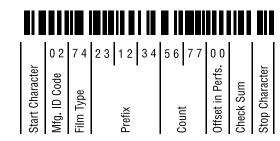
Encoded in USS-128 Bar code
