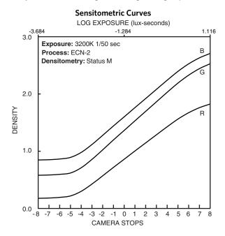
**Note:** The exposure scale for VISION3 Films is longer than previous VISION and VISON2 Films. Because of the extended highlight latitude we have expanded the exposure scale from a 0-4 increment to a 0-5 scale. In addition to the longer exposure scale, we are plotting 21 steps instead of 20.
