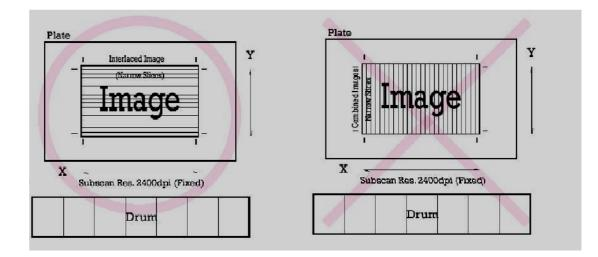
Due to the image direction restriction above, the maximum plate size that can be imaged may also be limited. For example, an 8u-up CTP cannot handle the largest plate size in the portrait direction.
