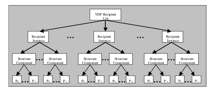
A structure component must have the same page layout and medium (substrate) type. For example, if the front cover and body pages have the same layout but different media, at least two structure components are required: one for the front cover, and another for the body.
