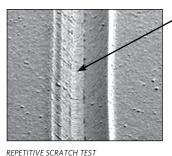
KODAK Photoplotter Film APR7 NO BREAKTHROUGH AFTER FOUR PASSES
