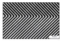
TOP VIEW Note: Small particles in the clear area are 1-3µm optically clear matte beads for improved vacuum contact.
