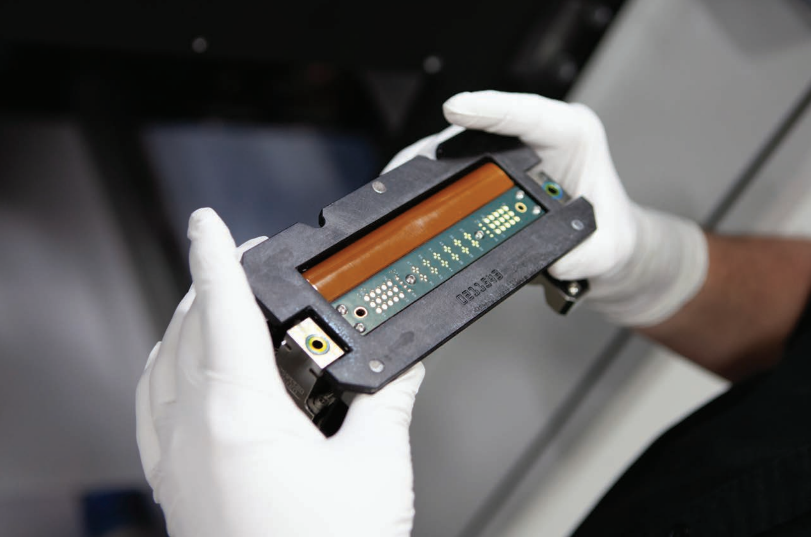
Stream jetting module used in PROSPER S-Series, PROSPER Plus, PROSPER 1000, 5000, 6000 and EVO M presses
