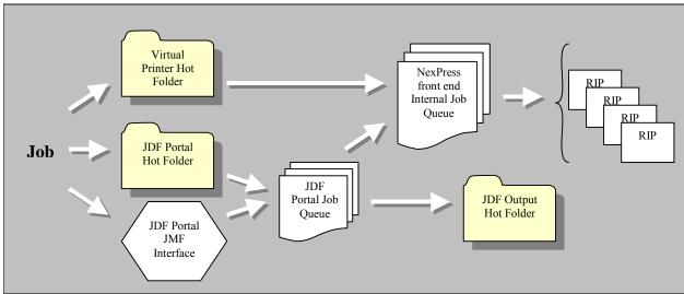
Regardless of the submission interface, all jobs are placed into the Internal Job Queue for processing. Jobs in the Internal Job Queue are referred to as Internal Queue Entries. Internal Queue Entries are RIPped and printed in the order of their arrival. Because job processing capabilities overlap within the NexPress front end, multiple jobs will execute simultaneously depending upon the availability of processing resources.
