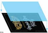
Metallic Clear Dry Ink can be applied at the press level as an adjustable uniform layer on the entire page. Four other coating modes are also available.
