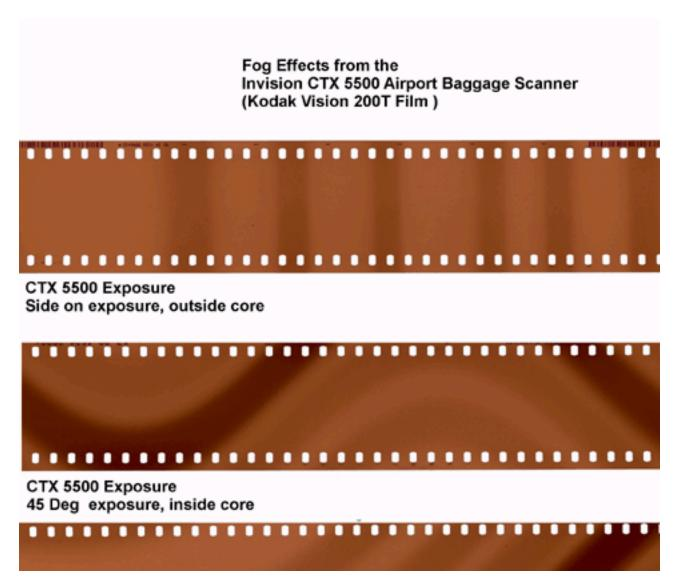
Below are samples of KODAK VISION 320T Color Negative Film (16 mm motion-picture film) exposed to an INVISION CTX-5500 baggage scanner.
