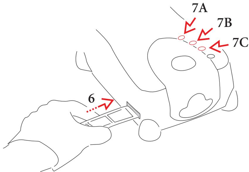
6. Gently move the filmstrip into the scanner from the left until the scanner detects the film and pulls the film into the scanner.
