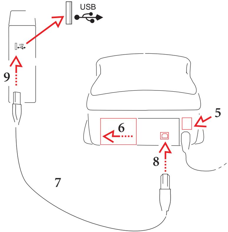
6. Slide the cover on the back of the scanner to the left to reveal the USB port.
