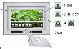
NOTE: When screen icons appear, LEDs turn on at touch-sensitive points along the raised guide.
