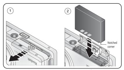
For information on replacing batteries and extending battery life, see page 59.
