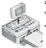
2 Place the camera on the printer dock. Push down to seat the connector
