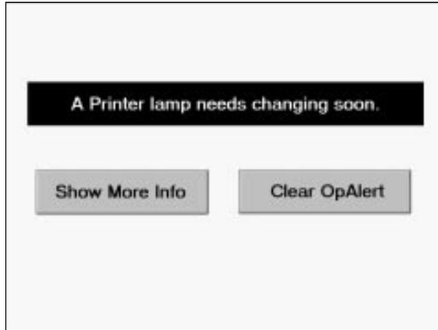
These Operator Alert messages are displayed if the processor is in Sleep Mode, Standby Mode, or Processing Mode. If you are in Processing Mode, continue to process your customer's films. You can change the filters/lamps when you go to Sleep Mode at the end of the day.
