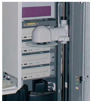
RIMAGE writers not only automatically load, record and stack discs but even print the label
