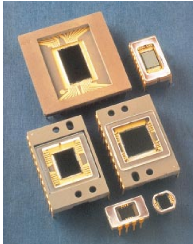
FIGURE 1. Historically, the optical format value for a CCD derives from the days when Vidicon vacuum tubes were used as sensing elements in television cameras. A 1-in. vidicon tube approximately 1 in. in diameter has a photosensitive area with a diagonal of 16 mm (about 2/3 in.). A CCD with a 16-mm diagonal is thus called a 1-in. CCD. Eastman Kodak makes interline CCD sensors in a variety of sizes.
